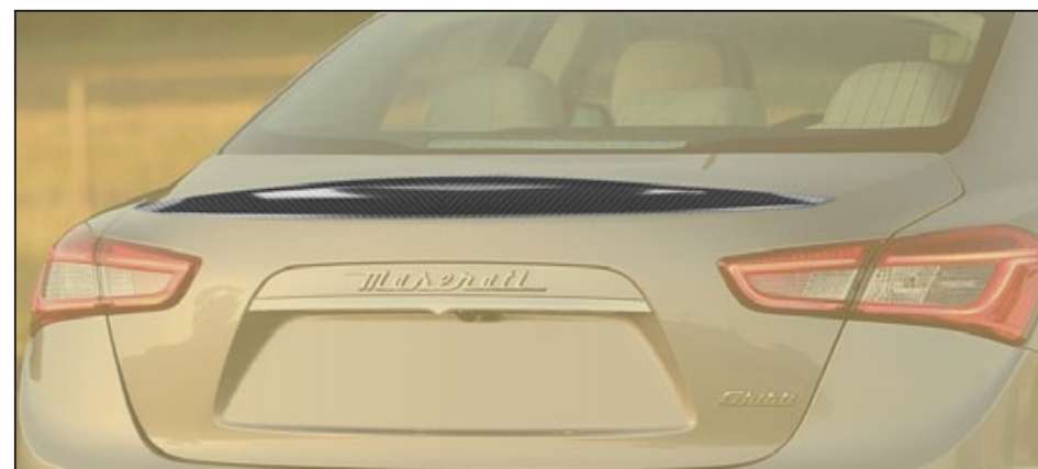
Rear deck lid spoiler - carbon 57X 830 841 visible carbon fibre primed without clear coat Rear deck lid spoiler - primed 57X 830 845 primed not visible carbon fibre
