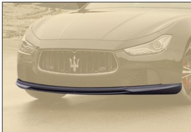
Front lip 57X 102 121 visible carbon fibre primed without clear coat
